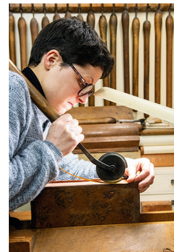
Clockwise from top center: Atelier Devauchelle, a notable Parisian book-binding workshop, in the morning hours; Naïk Duca uses a thin heated roller to press gold lines from foil; the shop's brass stamps, which are used to emboss patterns onto leather-clad books; restoring a volume of an 18th-century scientific dictionary.
