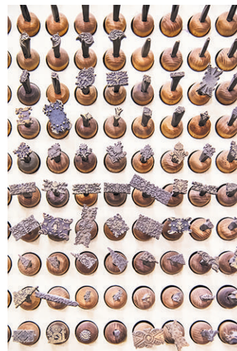
Clockwise from top center: Atelier Devauchelle, a notable Parisian book-binding workshop, in the morning hours; Naïk Duca uses a thin heated roller to press gold lines from foil; the shop's brass stamps, which are used to emboss patterns onto leather-clad books; restoring a volume of an 18th-century scientific dictionary.
